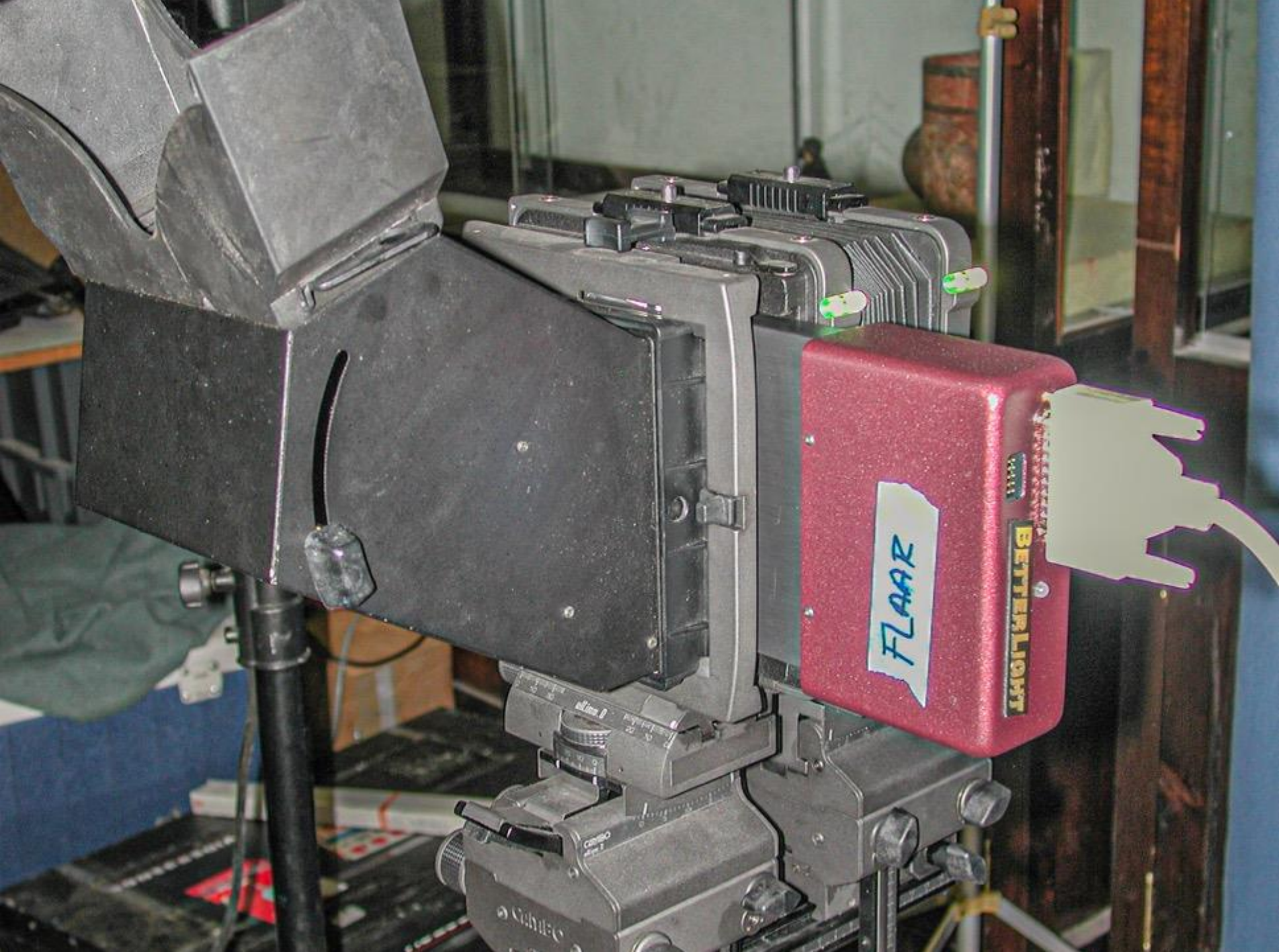
Fig. 192. As you can see in this photo, the Better Light scan back is inserted in an incredible Made in Germany Linhof 4x5" camera.
