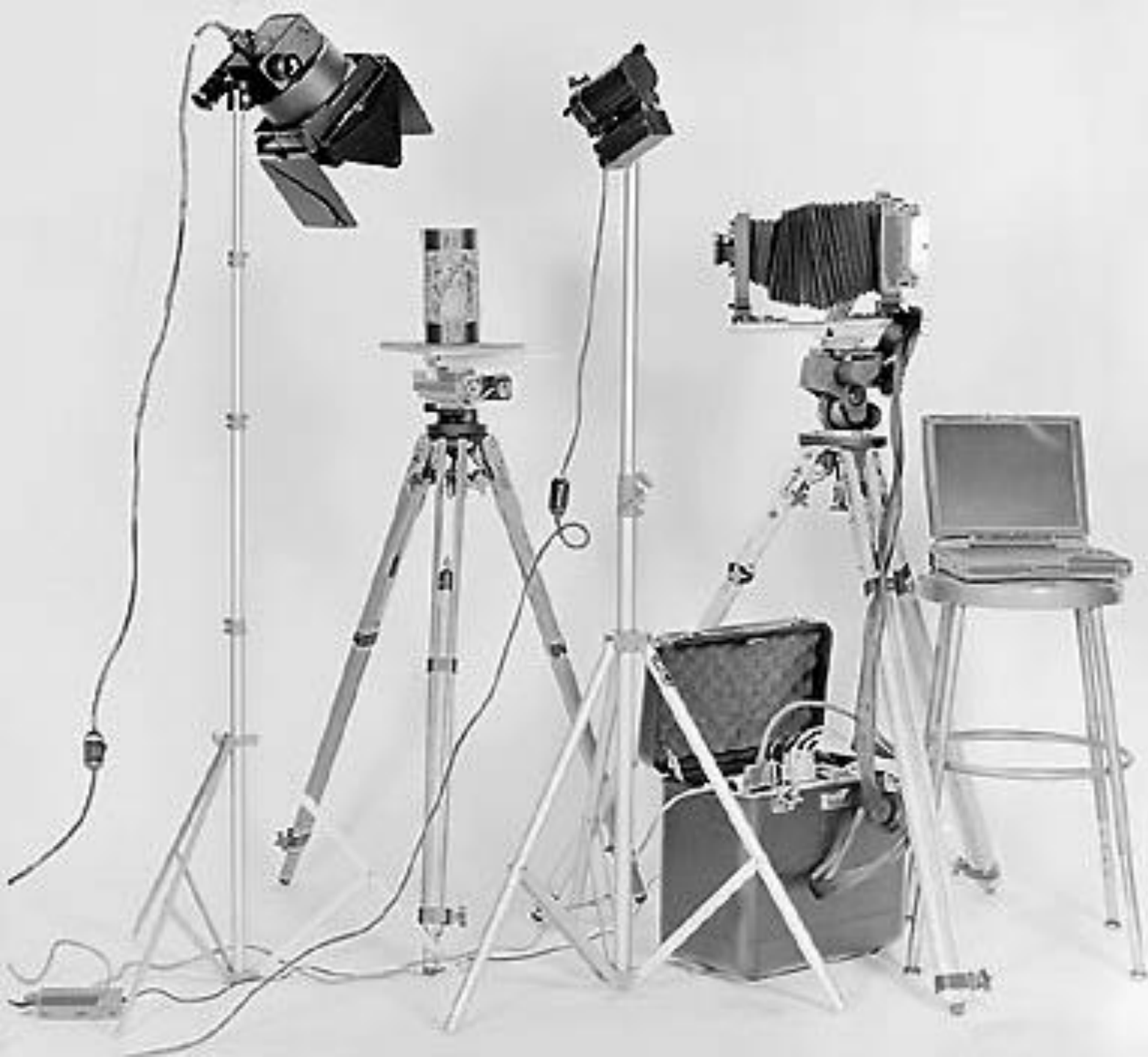
Fig. 195, a and b. This is an example of the complete studio (at the right): Mac laptop computer, metal suitcase filled with the Better Light computing system and software, one tripod and tripod head for the 4x5" camera. Another tripod for the Better Light turntable to hold the vase. Lights from each side.
