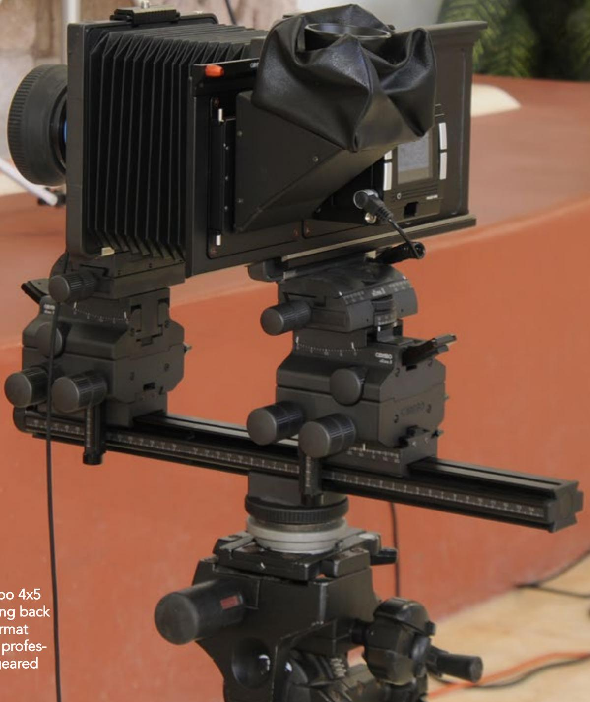
This is the reliable Cambo 4x5 view camera with a sliding back system for a medium format digital back. Notice the professional sized Manfrotto geared tripod head.
