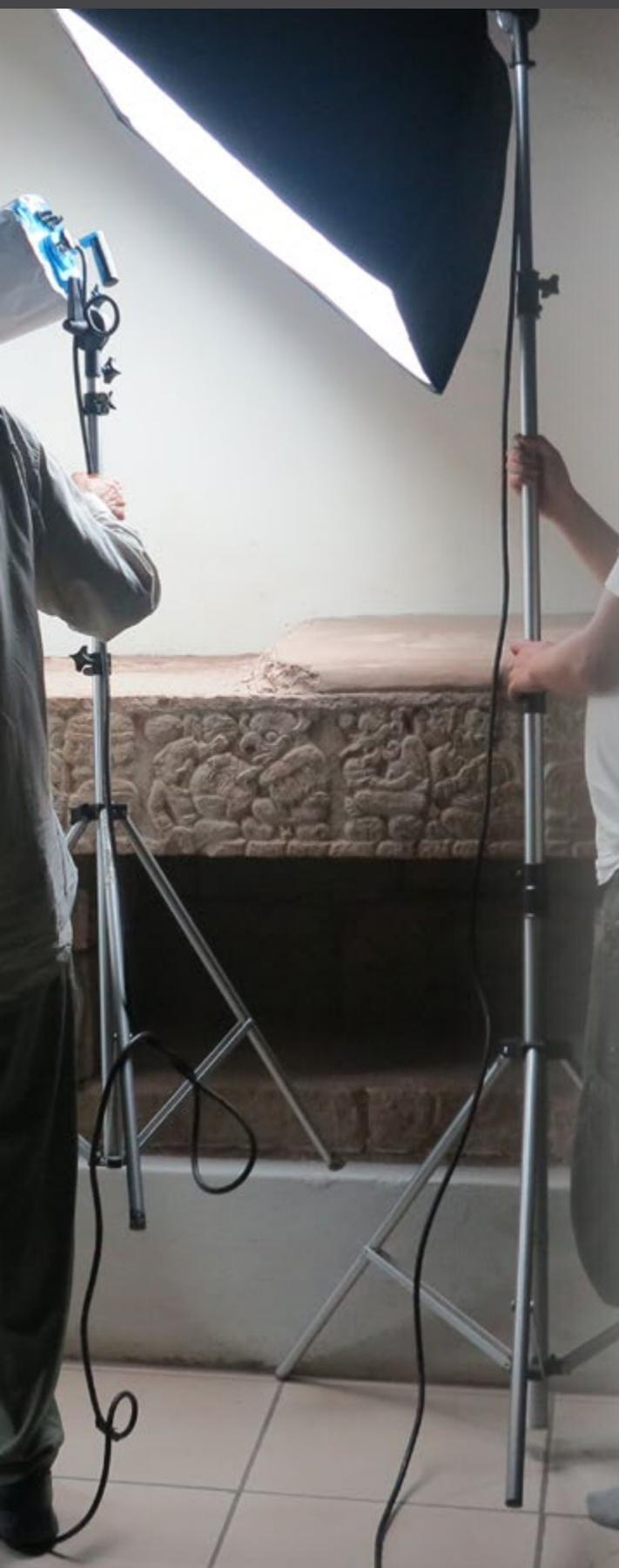
The advantage of the Spiderlite TD6 is that you can use either daylight fluorescent or tungsten halogen lamps.
